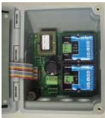
Figure 1.4 Two ISO-MOD I/O Modules Installed
